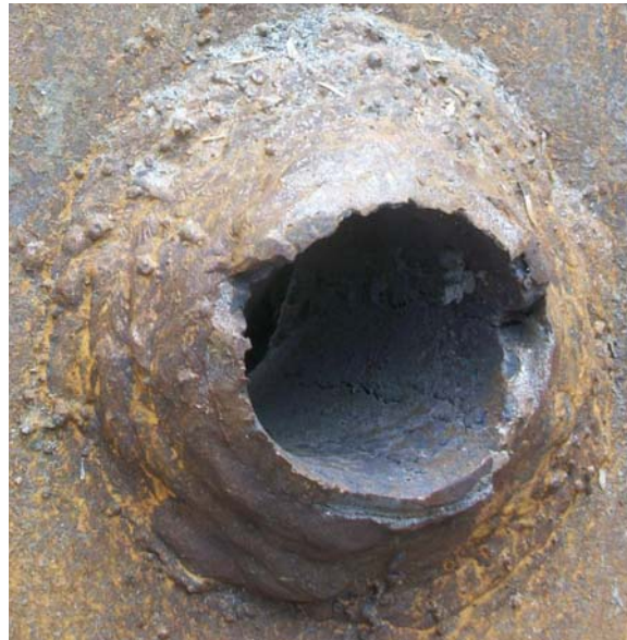
Photo 4 & 5: The feed water inlet stub to shell is seen without a sleeve pipe. This had led to cracks development due to cyclic thermal stresses. However the shell plate did not fail due to this crack as it is seen to be intact with main shell nearby.
