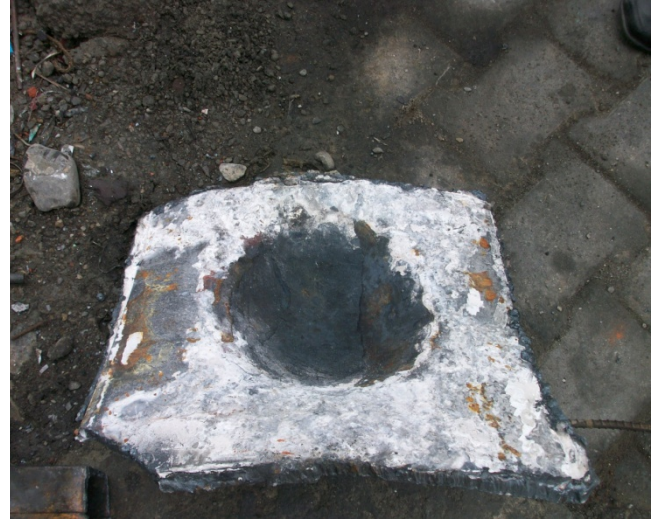
Photo 2: The back side (water side) of the bulged plate, showing scales (second time).
