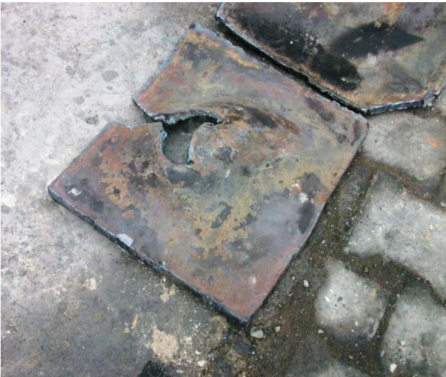
Photo 3: Part of the furnace shell that bulged first.
