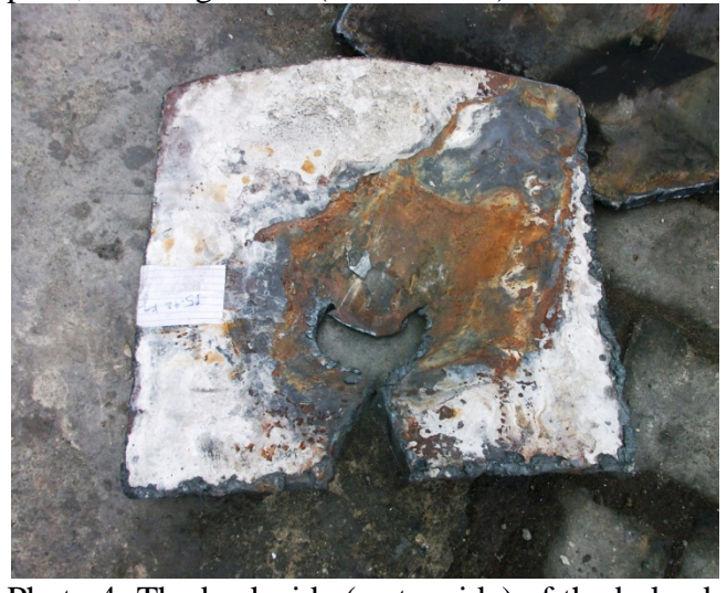
Photo 4: The back side (water side) of the bulged plate showing the scales (first time).
