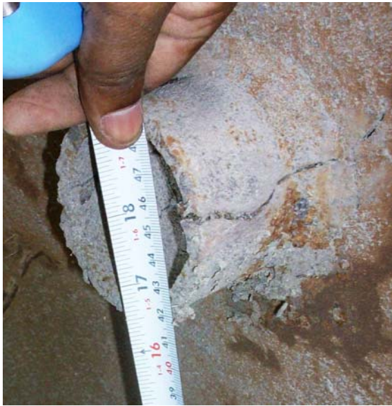
Photo 4 & 5: The feed water inlet stub to shell is seen without a sleeve pipe. This had led to cracks development due to cyclic thermal stresses. However the shell plate did not fail due to this crack as it is seen to be intact with main shell nearby.
