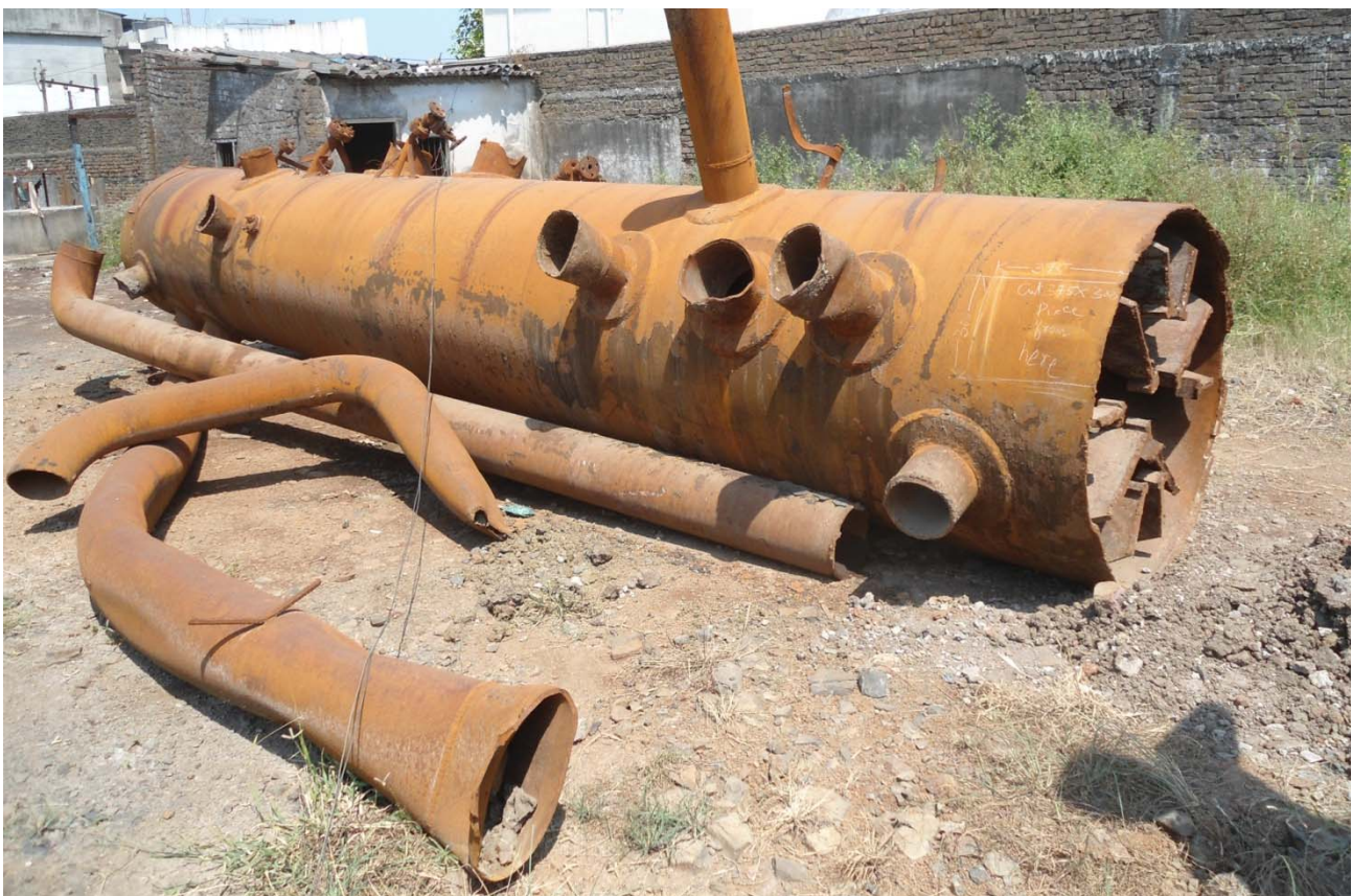
Photo 1: The steam drum was inspected at manufacturer's storage yard. It is seen that the flat ends are provided for the steam drum, instead of dished ends. The flat end had come off from the steam drum, which had led to this incident.
