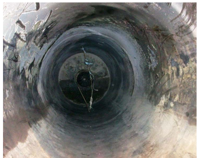
Photo 6: Burner air flow test. It showed less air flow at bottom when tested with flags.
